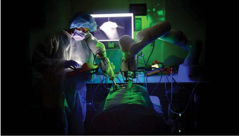
Figure 8.4 Image of smart tissue autonomous robot during preparation for intestinal anastomosis procedure. From E. Svoboda, Your robot surgeon will see you now, Nature 573 (Sept), 2019, S110–S111.
